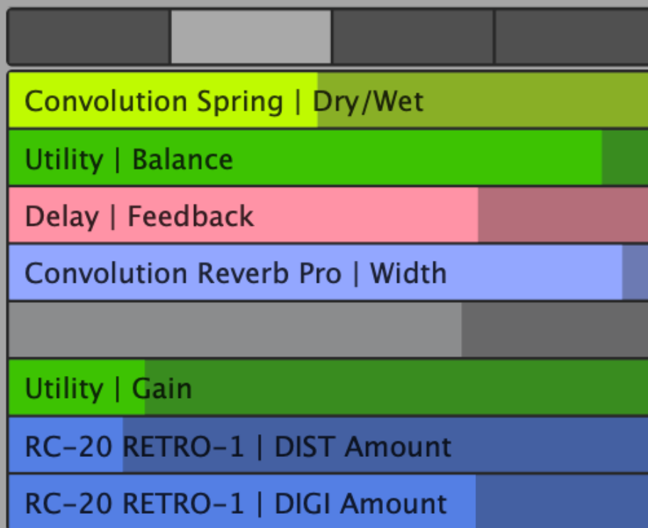
Figure 7.1 The channel lanes in the Survey interface display mapped parameters and their values for the selected stage. The color of the channel lane reflects the track containing its mapped parameter.
